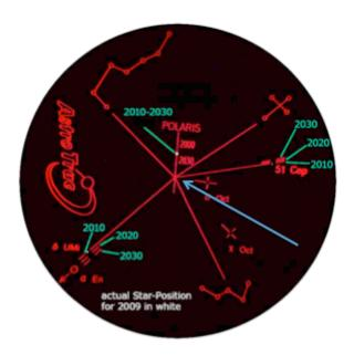
Here is what the actual physical reticle disc inside a polar scope looks like. This one is from an Orion polar scope:
