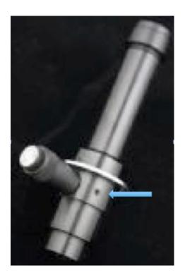
The three (3) screws are spaced 120 degrees apart. Working with these screws requires a tiny metric allen wrench and is virtually impossible. We need to replace these screws so we can make adjustments quickly and easily using only our fingers.
